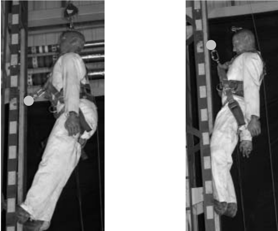
Figure 92 ATD just before release (left hand view) and in post-drop suspension (right hand view)
