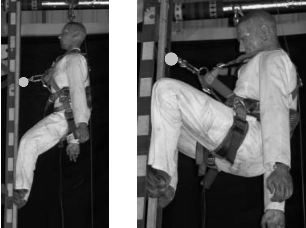
Figure 94 ATD just before release (left hand view) and in post-drop suspension (right hand view)
