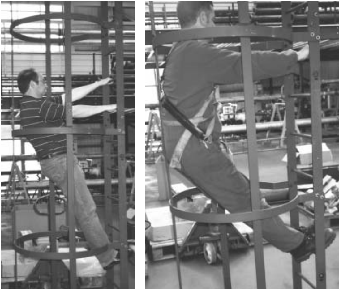
Figure 33 Example of how taller person with relatively long reach and leg length (right hand view) can lean back against cage with grip maintained as compared to smaller person (left hand view)
