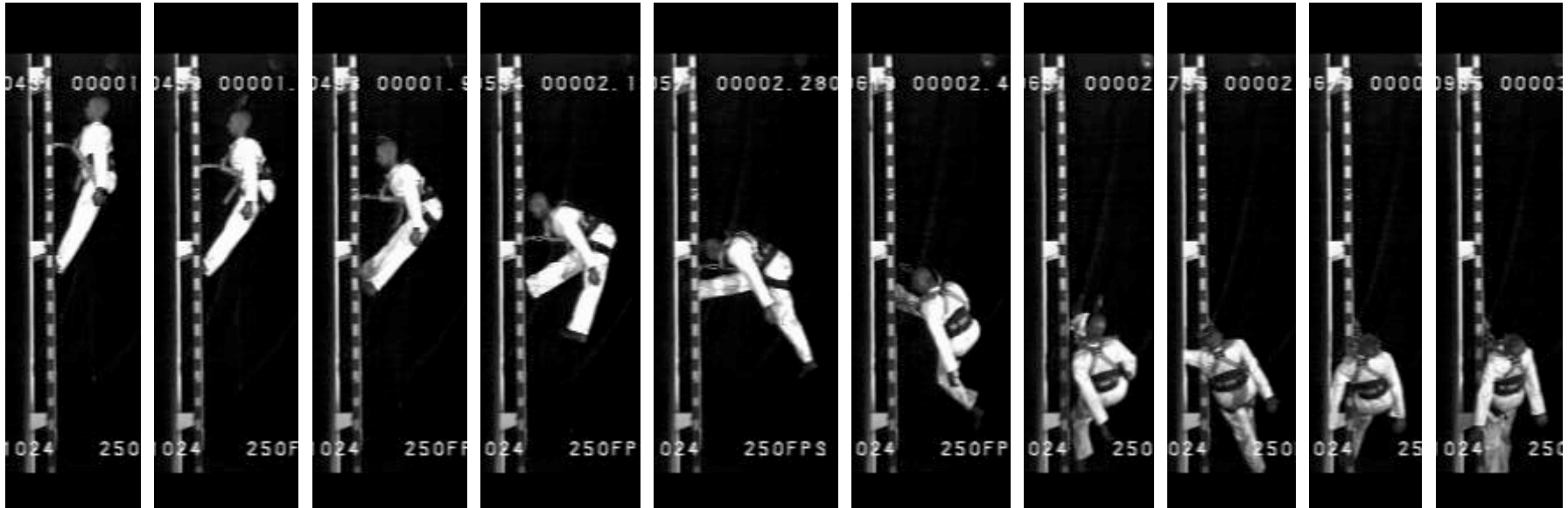
Figure 83 Kinematic sequence of ATD fall trajectory from test 13 (FAS 3)
