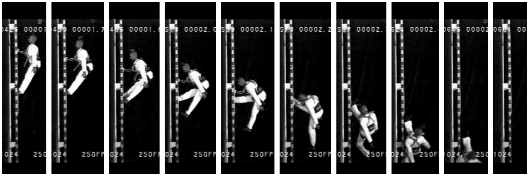
Figure 80 Kinematic sequence of ATD fall trajectory from test 12 (FAS 2)
