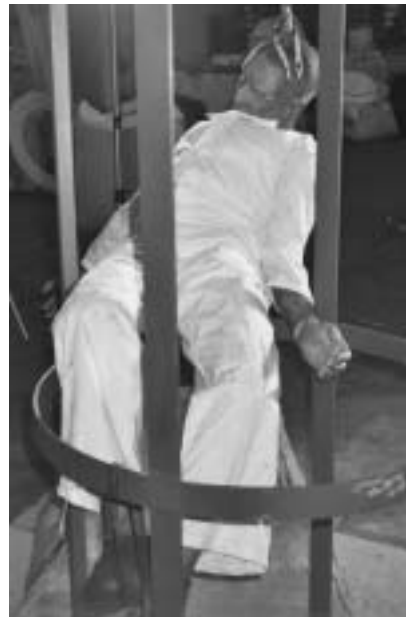
Figure 29 Three views of test dummy being slowly lowered to simulate fall through cage aperture
