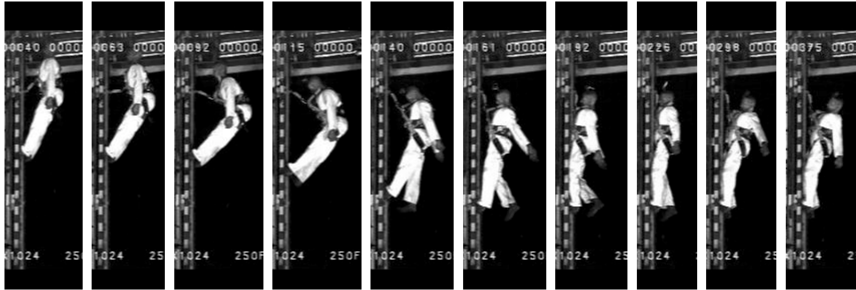
Figure 89 Kinematic sequence of ATD fall trajectory from test 15 (FAS 4)
