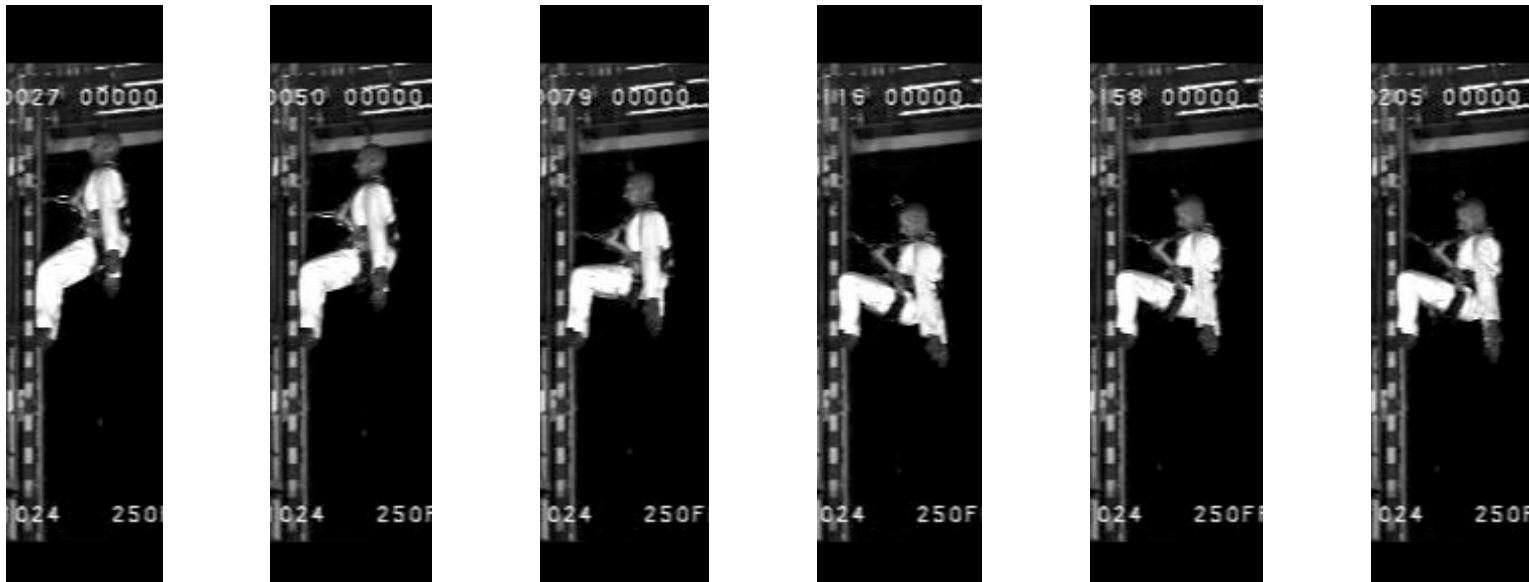
Figure 95 Kinematic sequence of ATD fall trajectory from test 18 (FAS 5)
