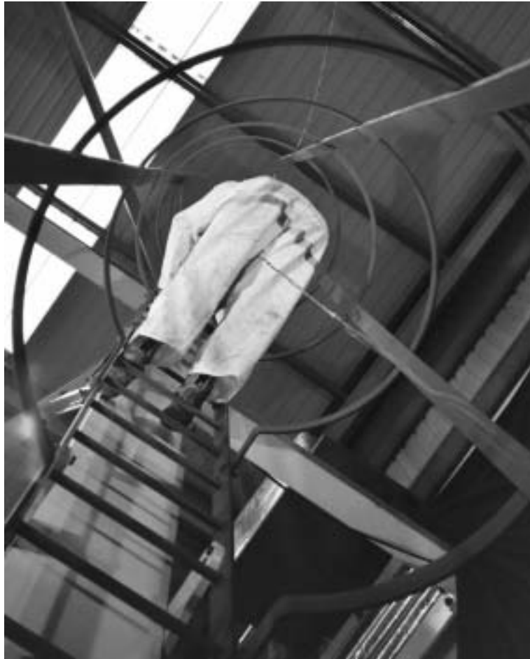
Figure 37 ATD in pre-release position inside caged ladder; accelerometer cables can be seen hanging from ATD's posterior
