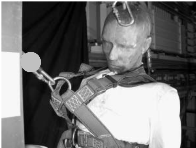
Figure 96 Example of harness stretch
